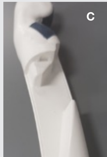
Figure 1. Examples of surface features of ultrasound probes: an orientation marker located on the side of the probe body (A); grooves to assist with grip (B); notch for attachment of needle guide (C).
