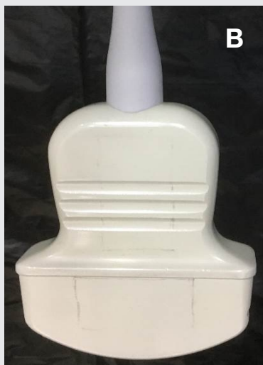
Figure 1. Examples of surface features of ultrasound probes: an orientation marker located on the side of the probe body (A); grooves to assist with grip (B); notch for attachment of needle guide (C).
