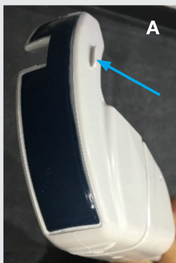
Figure 1. Examples of surface features of ultrasound probes: an orientation marker located on the side of the probe body (A); grooves to assist with grip (B); notch for attachment of needle guide (C).
